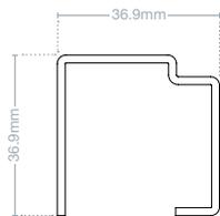
Heavy duty sash reinforcement
