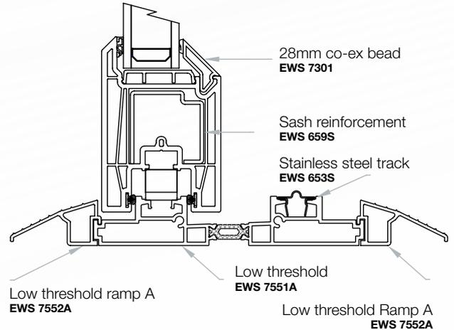
VERTICAL CROSS SECTION THROUGH SLIDING SASH WITH LOW THRESHOLD
